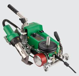
The user-friendly, automatic welder UNIPLAN 500 has even more welding power and advantages than the UNIPLAN 300. It is perfect for welding taped seams, hems and piping on truck tarpaulins, tents and billboards.
