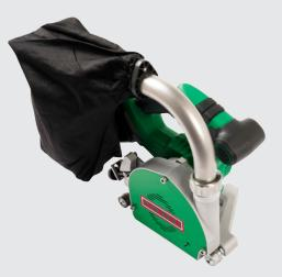
The GROOVER 500-LP battery-operated grooving machine mills grooves for welding seams when laying resilient plastic and natural floor coverings such as linoleum and rubber. It's cordless, uses a general-purpose milling cutter and works quickly.
