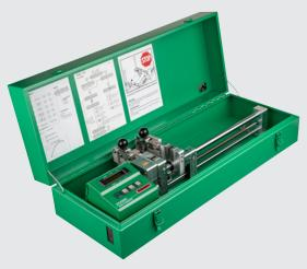
The EXAMO 300F USB is the ideal testing device to check welded membrane seams for peel adhesion, tensile strength and shear strength - tested and proven worldwide.
