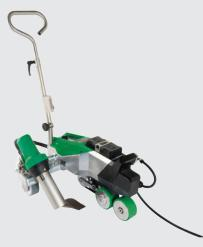
The VARIMAT 500 automatic welding machine offers reliability in flat roof welding. High contact pressure, innovative nozzle swivel-in mechanism and variable transport axis ensure welding quality. Convertible from 230 to 400 V.
