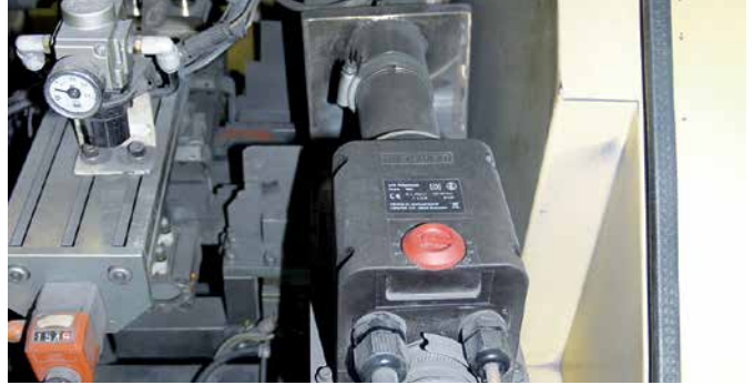
Deflashing foil sleeves from charcoal filter elements
