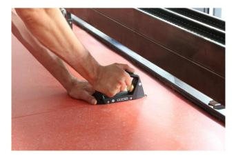
With the GROOVY handheld gouging tool, the beginning and the end of a groove can be completed up to last millimeter.
