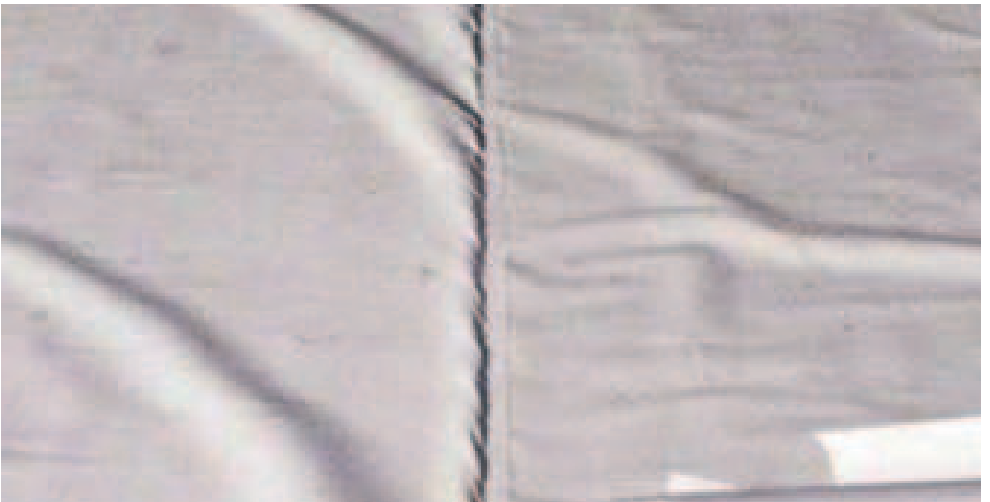
Typical wave and wrinkle formation at excessive welding temperatures. The welding temperature must be reduced to prevent wave formation!
