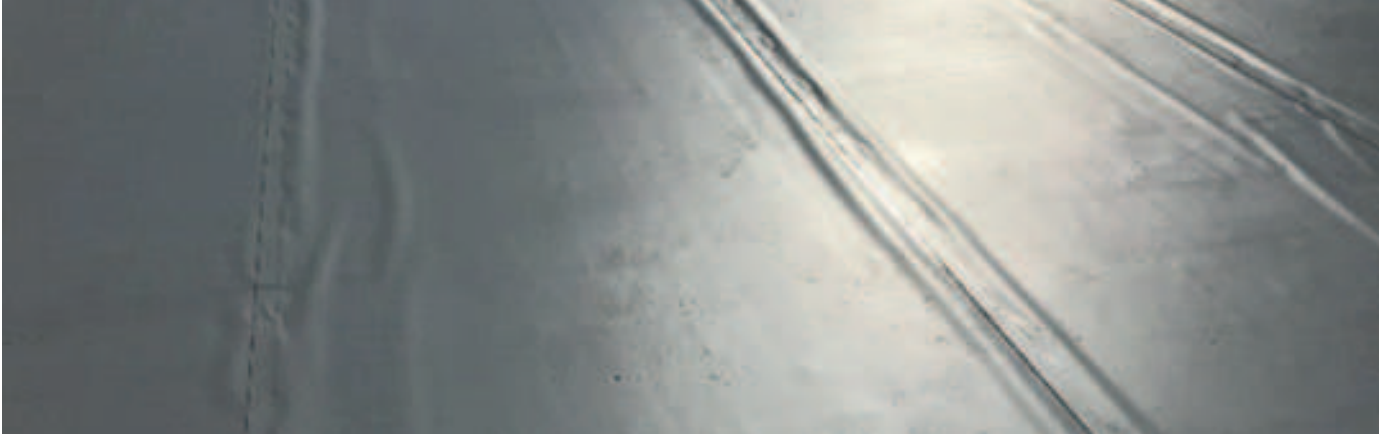
Typical weld with wave formation and wrinkles at excessive welding temperatures
