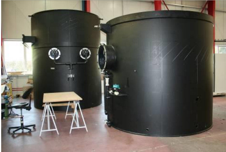
Storage tank Polyethylen (HD-PE)
