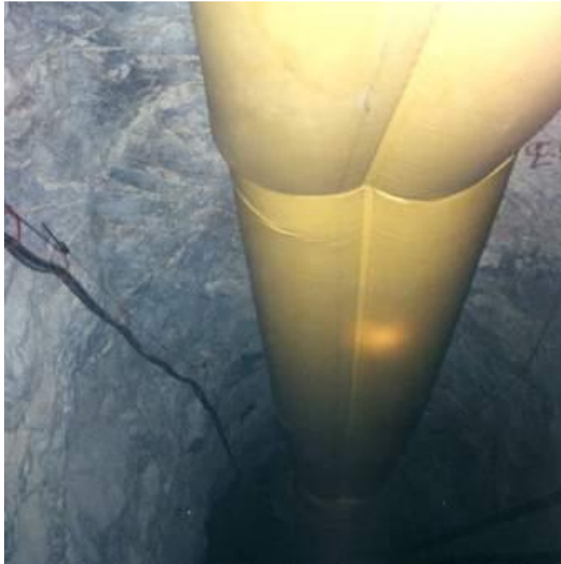
Ventilation tubes welded with UNIPLAN E and VARIANT T1
