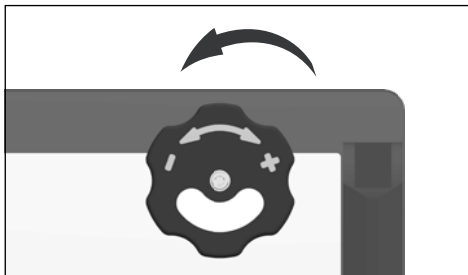
Turn anti-clockwise (-) pressure setting valve open/minimum pressure
