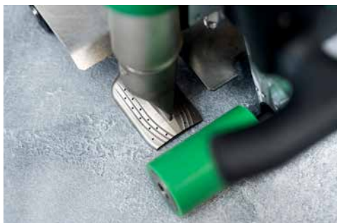
Simultaneous butt welding on seam tape
